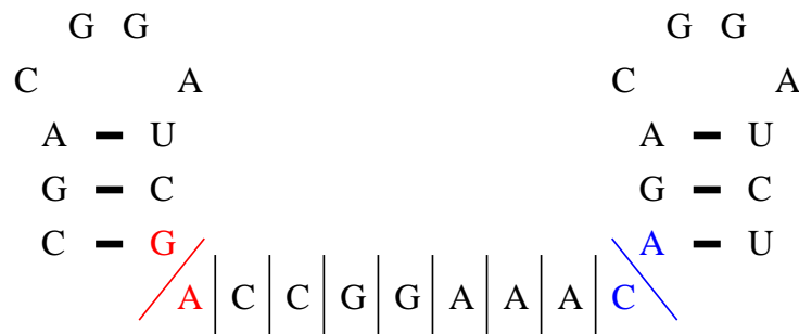
Figure 2.11: Bifurcation constraints. When two substructures are joined, there are usually many exactly similar ways to do it (The figure shows a single sequence example for clarity). In the figure ten slightly different pairs of substructures can all be joined into the same structure. FOLDALIGN therefore only calculates this structure once. In version 2.0 the pair of substructures separated by a red line is used. In 2.1 the substructure pair separated by the blue line is used. Limiting the bifurcation to the blue pair instead of the red pair allows the memory requirement to be lowered since it is only necessary to store subalignments which end with a base pair for the positions upstream of the current position.
