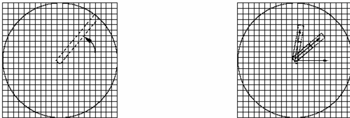
Figure 12. Radial average and angular average of Fourier power spectrum.
