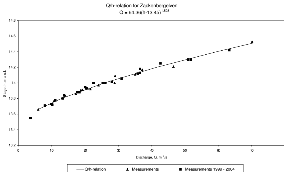
Figure 2.12. Water level – discharge relation curve (Q/h-relation) for Zackenbergelven at the hydrometric station, 1995-1998. The coefficient of correlation ( R^2 ) for the curve is 0.99. Measurements from the period 1999-2004 indicate that no major changes have occurred to the river profile since 1998.
