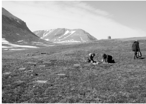
Figure 5.4. Vaccinium Canopy Experiment. Field manipulation of ambient UV-B by means of filter screening close to the Zackenberg Research Station.
