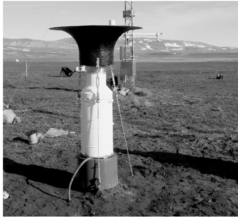
Fig. 2.2. The new foundation of the Belfort precipitation gauge that elevates the measuring device above the ground and thereby hopefully reduces problems with freezing water around the equipment.
