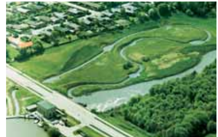
Fish ladders (top picture) are often only passable for species that are strong swimmers. Bypass streams, on the other hand, extend the water drop over a longer reach and are therefore more often passable to all species of fish and invertebrates. The lower picture shows the 655 m-long bypass stream at the Holstebro hydroelectric power station on the River Storå.
