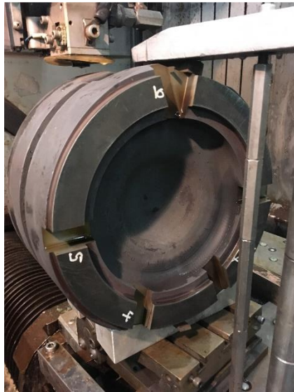
Figure 10.1: An ex-service wedge gate valve.
