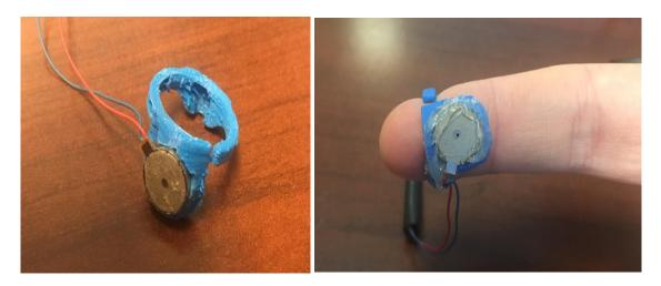
Figure 2.3: 3D Printed Ring Holding Linear Actuator
