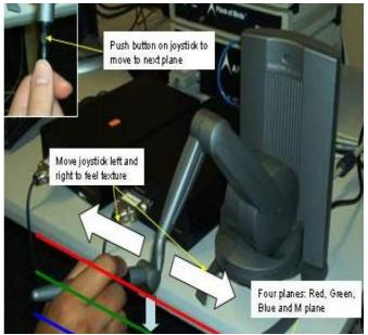
A joystick that provides tactile force feedback to users as the virtual map is searched. The device is created by SensAble Technologies (Kahol et al, 2006)
