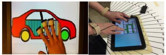
Examples of using wearable tactile systems to search virtual tactile maps, the left image shows a person wearing optical sensors to detect color to provide tactile feedback (Burch and Pawluk, 2011). While the right image uses an app to detect the RGB value the finger is over and provide tactile feedback to the finger through tactile rings worn by the user (Adams et al., 2015).
