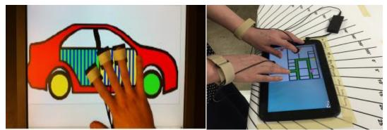
Burch and Pawluk (2011) allows for the use of multiple optic color sensors to search images to provide feedback to the fingers. While Adams et al. (2015) provides two tactile rings to allow the searching using multiple fingers.
