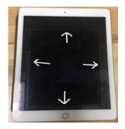
Figure 5.2: Android table with screen protector cut-out defining map edge
