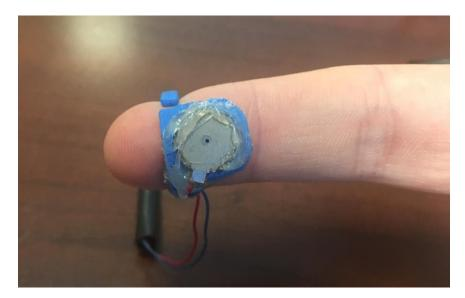
Figure 4.1: 3D Printed Ring Oriented Properly on the Index Finger
