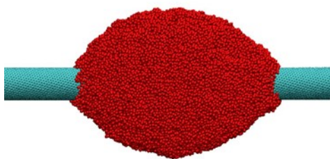
Figure 9: Equilibrium barrel shape of atomistic droplet on a fiber with r_f = 12.8 \text{ \AA}
