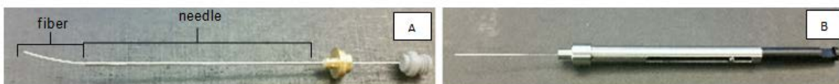
Figure 2. SPME fiber assembly: (A) the exposed fiber inside the SPME fiber assembly; (B) the holder assembly used for injection onto the GC.
