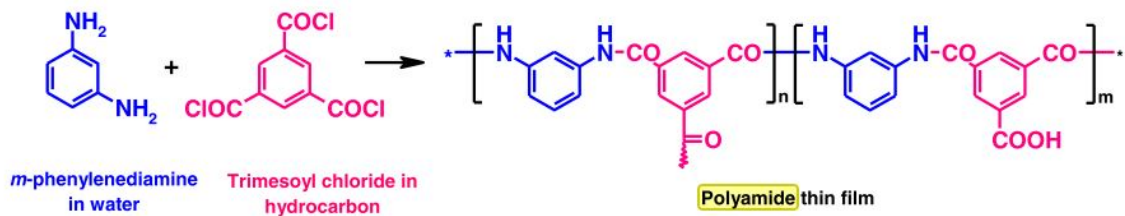
Figure 3.6: Interfacial polymerization for thin film composite membranes.
