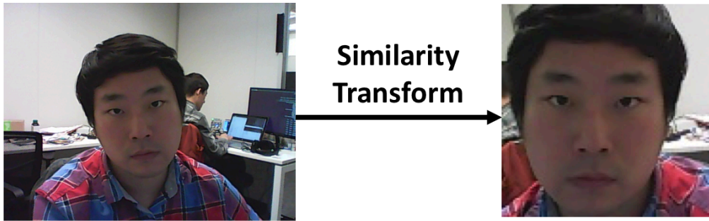
Figure 13 Example of a similarity transform. The right image contains a face that was rotated, after similarity transform, the resulting face in right image is rotated back to the frontal face orientation.
