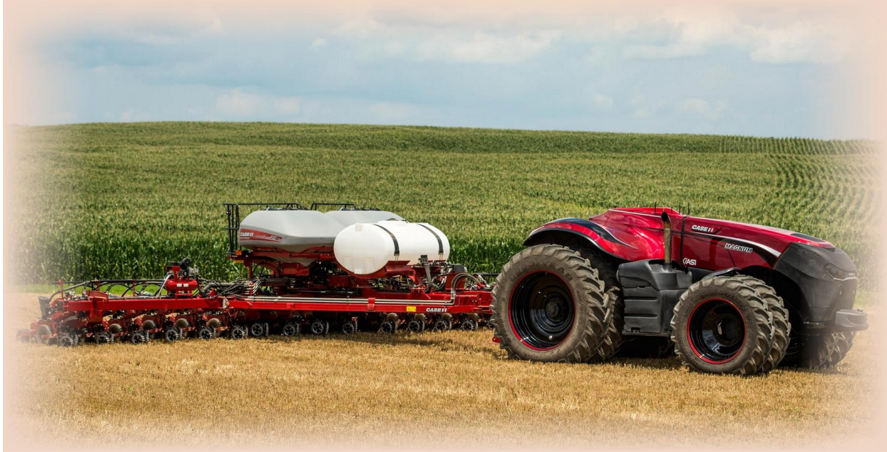
Figure 3. Case IH Magnum Autonomous Tractor in field with a planter implement (from http://www.cnbc.com/2016/09/16/future-of-farming-driverless-tractors-ag-robots.html )
