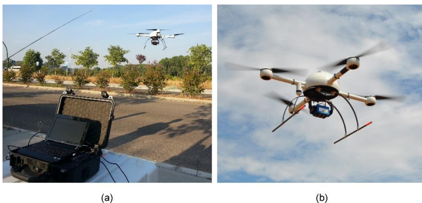
Figure 4.2 a) and b) UAV flying the study area equipped with the multispectral camera
