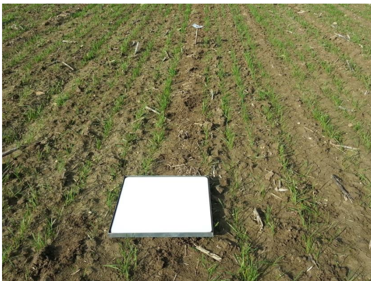
Figure 3.3 Details of experiment setup to assess spectral discrimination: Spectralon panel placed in the middle of the study area.
