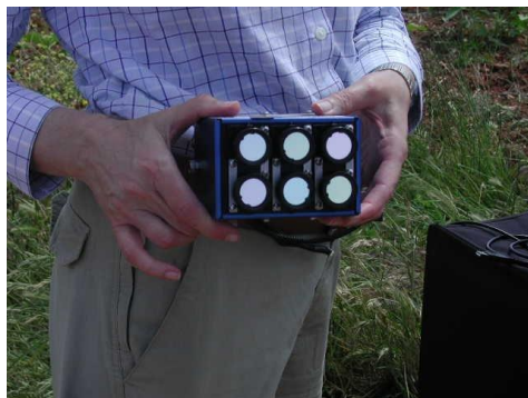
Figure 4.3. Multispectral sensor TetraCam Mini-MCA: Distribution array of sensors.
