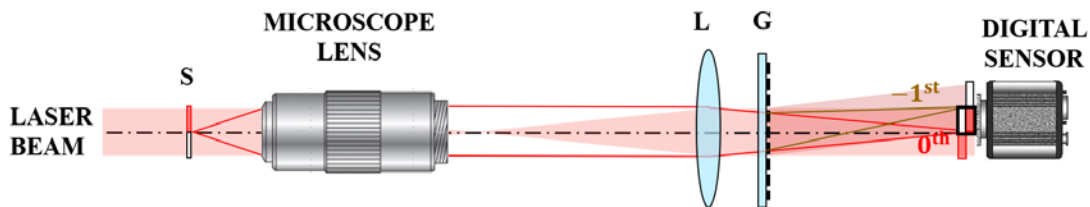
Figure 2.11. DHM layout working in a transmissive imaging mode.
