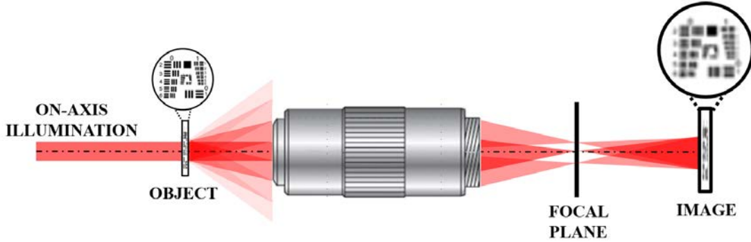
Figure 2.15. Imaging through an optical system according to Abbe's theory.
