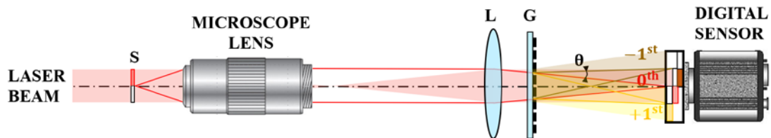
Figure 2.6. Scheme and ray tracing of a CPI based on a diffraction grating employed in DHM . S, L, and G denote sample, lens, and 1D diffraction grating.
