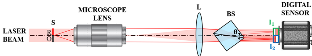
Figure 2.7. Scheme and ray tracing of a DHM layout based on a BS cube interferometer.
