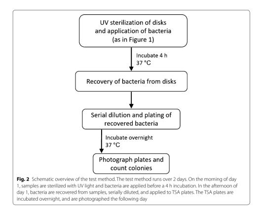
each series was applied to TSA plates, and evenly spread using a sterile disposable plastic cell spreader. Plates were inverted, and incubated overnight (18–20 h) at 37 °C.
