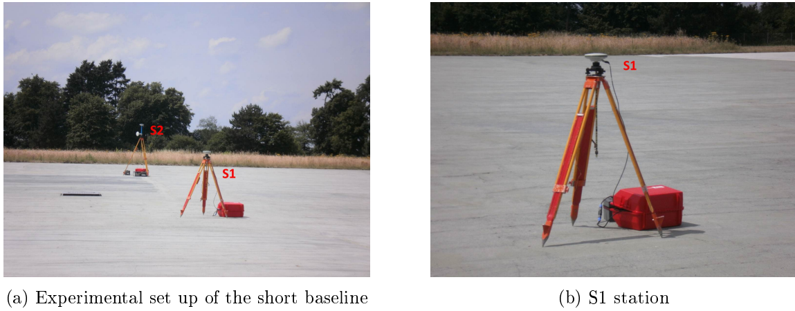
Figure 6.22.: Experimental set-up of the short baseline of the first experiment at PTB. S1 and S2 are the two antenna positions in a high-low set-up configuration.
