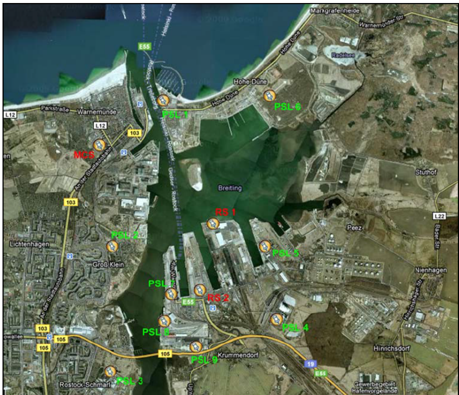
Figure 4.1.: Rostock harbour area and Sea Gate infrastructure consisting of nine pseudolites (PSLs) and the two monitoring stations (RS1 and RS2). Adopted from Dietz et al. (2010)
