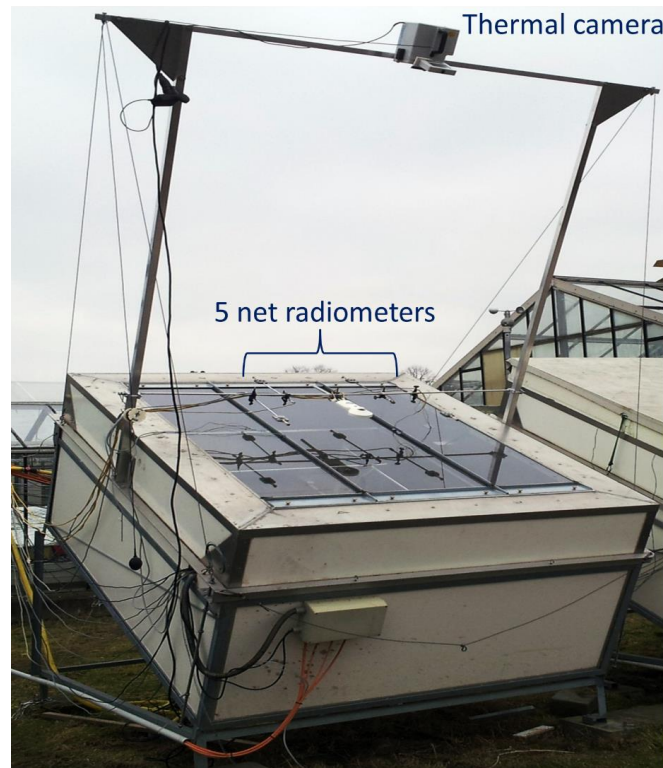
Fig. 4.5. South-facing thermal box for thermal radiation exchange measurements.
