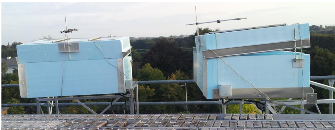
Fig. 4.16. An arrangement of the miniaturized thermal boxes oriented horizontally.
