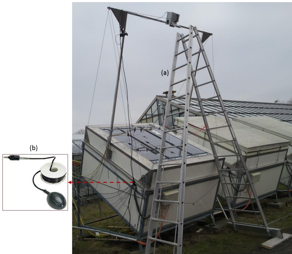
Fig. C6. Setup for mounting the thermal camera above the thermal box: (a) Ladder, and (b) Hama air bulb remote control release for capturing images.
