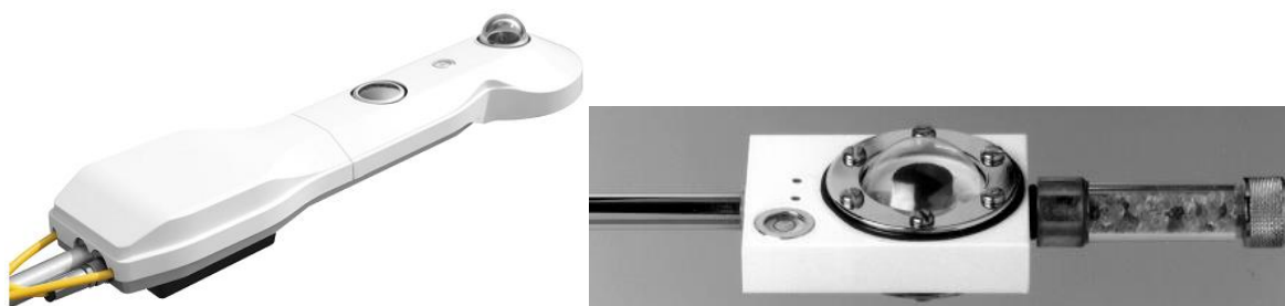
Fig. 4.6. CNR 4 (left) and 240-8110 (right) net radiometers used in thermal radiation exchange measurements (Sources: Kipp & Zonen, 2009; NovaLynx, 2013).
