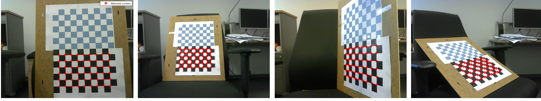
FIGURE 2.3: Examples of the checkerboard images; the detected corners are shown with red crosses.
