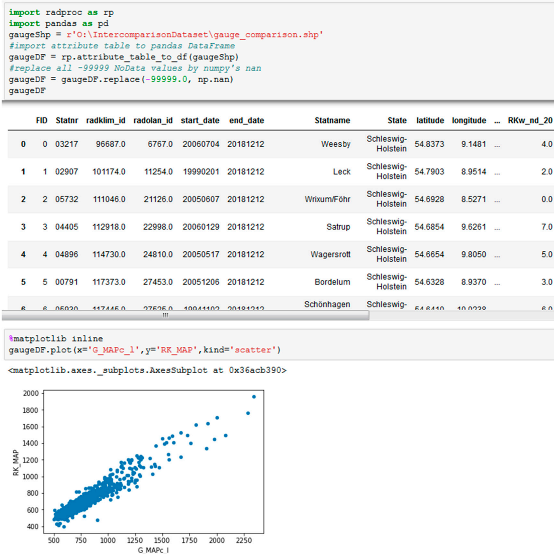
Figure 5. Importing the gauge shapefile into a DataFrame and plotting the mean annual precipitation sums of gauges and RADKLIM against each other.
