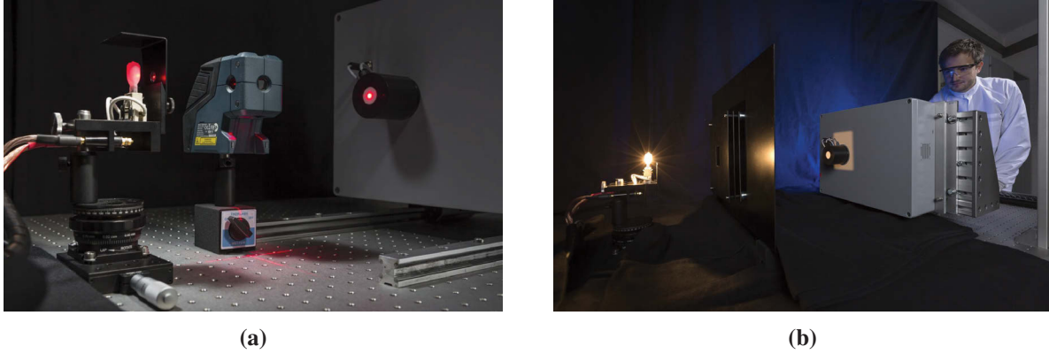
Figure 2.21: Setup for radiometric calibrations of spectrometer built up during this work. Figure (a) shows the alignment of calibration lamp and entrance optic of the spectrometer using a bidirectional adjustment laser. Figure (b) shows the adjusted setup during the irradiance calibration of the spectrometer.
