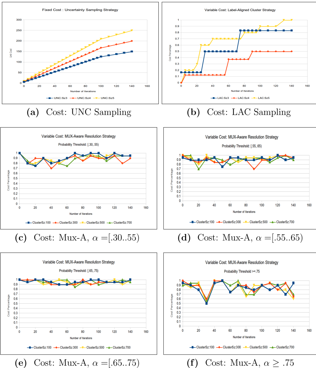
Figure 4.6 Fixed cost of basic uncertainty sampling strategy (4.6a); variable cost of using a strategy based on Labeling-Aligned Clustering (4.6b). Cost of global clustering with Mutual Exclusive-Aware strategy, for threshold probability, \alpha = , for: \alpha = [.30..55] (4.6c); \alpha = [.55..65] (4.6d); \alpha = [.65..75] (4.6e); and (\alpha \geq .75) (4.6f).
