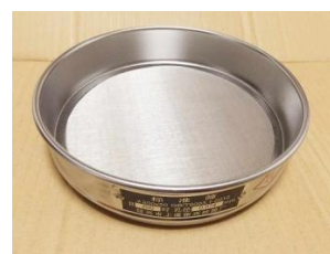
Fig. 3. GB / T6003.1-2012 sieve with a cell of 74 microns.
