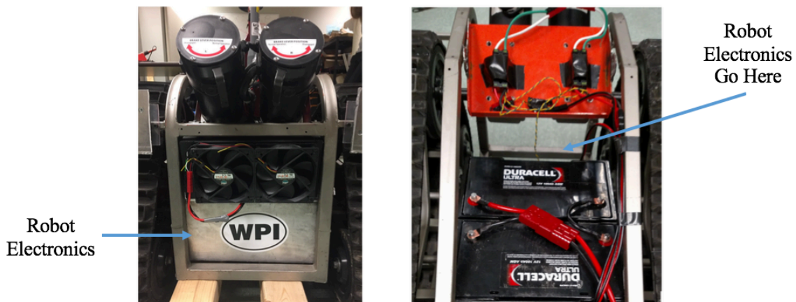
Figure 14: Batteries and Electronics Box This image shows the location of the robot electronics and how they are inaccessible due to the location of the batteries.
