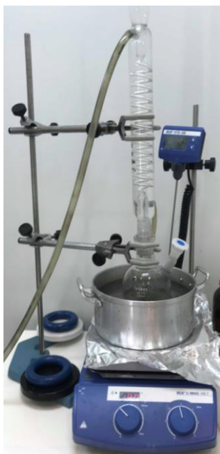
Figure 3. Bath and reactor used in the CWPO and H_2O_2 decomposition experiments
