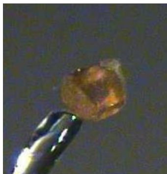
Figure 4.8. A: Diffraction quality pale-yellow crystal used for this analysis. B: ORTEP view of the Iron complex, ( S )- 9cc . Ellipsoids are drawn at 50% probability. Color code: O, red; C, blue; Fe, orange. H atoms are omitted for clarity.
