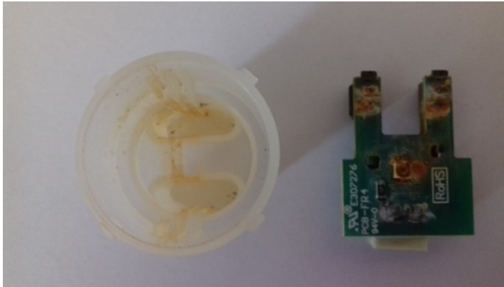
Fig. 4. The turbidity sensor when it starts displaying rust.
