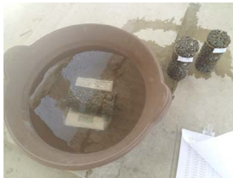
Fig. 2. Samples identified after weighing submerged in water
