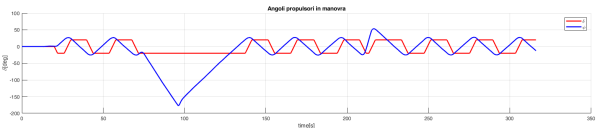
Fig. 10. The angle of thrusters ( \delta ) and the yaw angle ( \psi ) in the zigzag simulation
