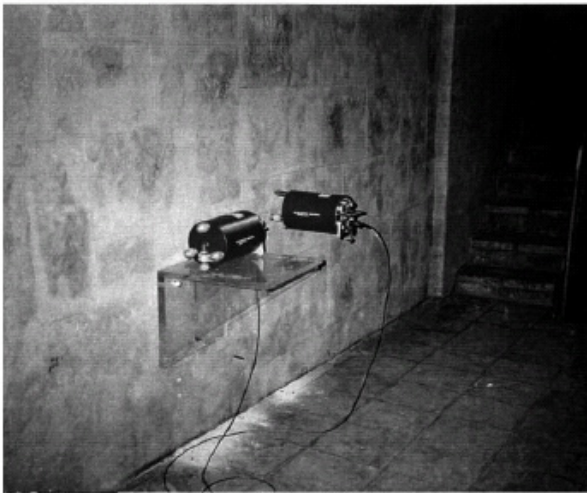
Fig. (6). Seismometers respectively fixed to a cantilever and the wall along two orthogonal directions.
