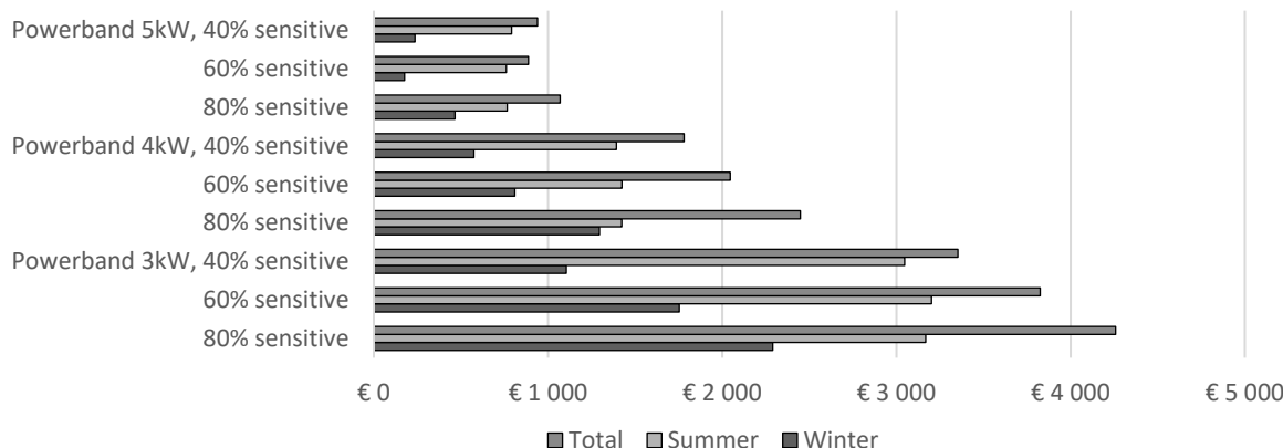
Figure VI-B Savings for LV cables in last year of simulation, by season, 'GG' scenario
