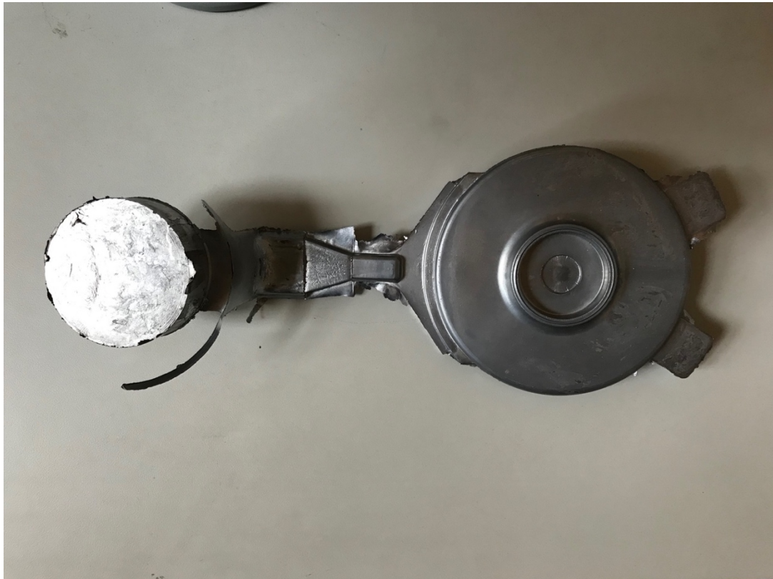
Figure 3-4 Casting of the Floor/Ceiling Plate with riser and feeder
