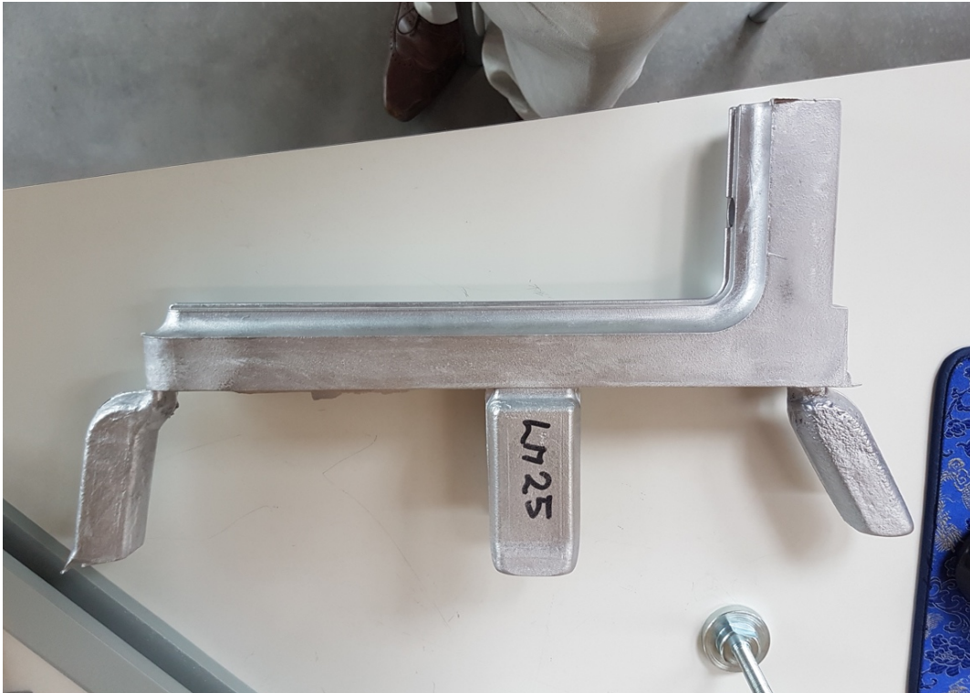
Figure 3-5 Casting of the Stabilising Foot with risers and feeder
