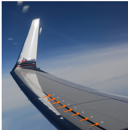
Figure 1.5: Vortex Generators on a Boeing 737-800 wing
