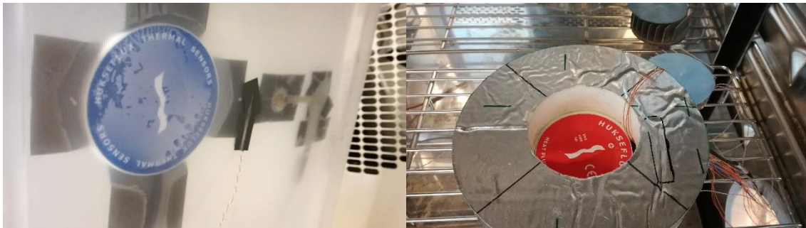
FIGURE 3. 7. THE TWO EXPERIMENTS THAT TOOK PLACE IN THE LABORATORY FACILITIES INVOLVING HUKSEFLUX SENSOR. ON THE LEFT, A TRANSIENT TEST WHERE THE BOX WAS KEPT AT 20 °C AND PUT INTO THE CLIMATE CHAMBER AT 10 °C. ON THE RIGHT THE HUKSEFLUX SENSOR WITHIN THE CALIBRATION ASSEMBLY.
