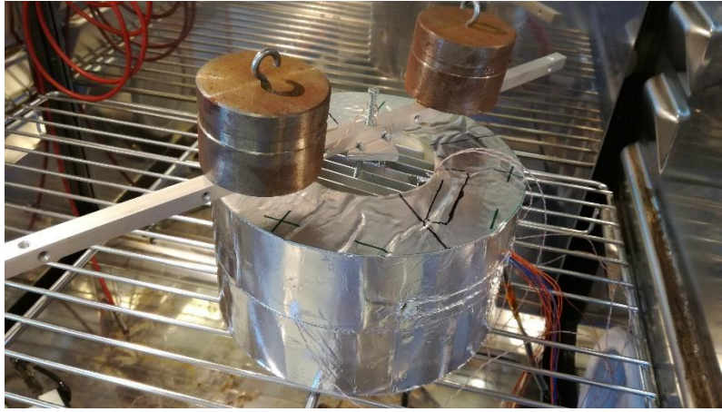
FIGURE 3. 4. WHOLE ASSEMBLY OF THE CALIBRATION SYSTEM WITH THE JIG INSIDE THE CLIMATE CHAMBER.
