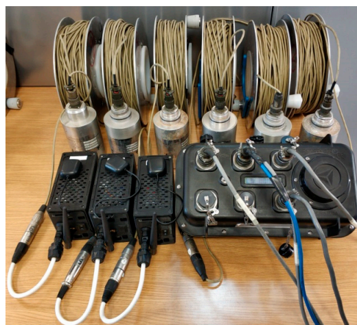
Figure 16. Mark L-4 sensors connected to the commercial equipment, Reftek, and the developed acquisition system, Geophonino-W.
