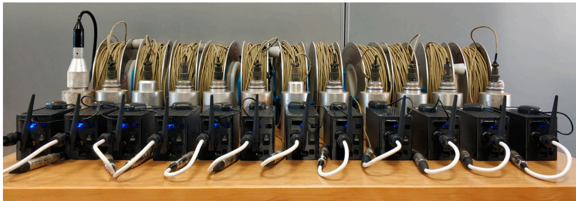
Figure 14. ACN modules connected to Mark L4 1 Hz sensors.
