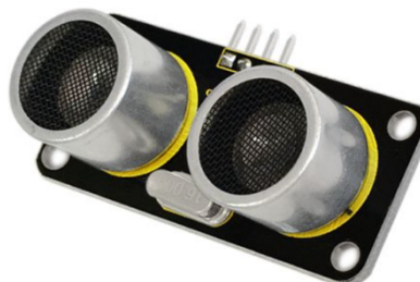
Figure 4.26. Characteristics of the Keystudio SR01. [36]
