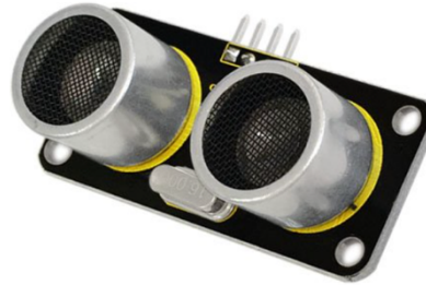
Figure 4.15. Characteristics of the Keyestudio SR01. [36]
