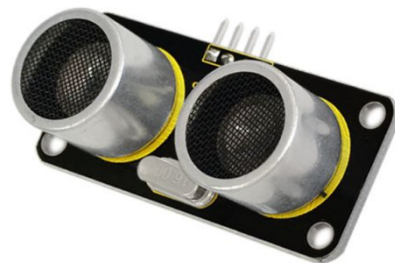
Figure 5.5. Characteristics of the Keystudio SR01. [36]
