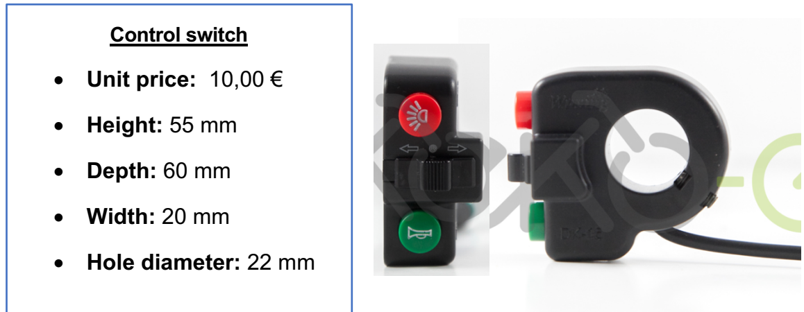
Figure 4.28. Characteristics of the control switch that will be incorporated. [37]
