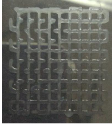
Figure 38. Dry printed structure.
