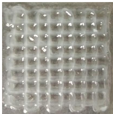
Figure 43. Printed structure of 4 layers in solution form and PBS addition, CS/ \beta -GP with blue nozzle.
