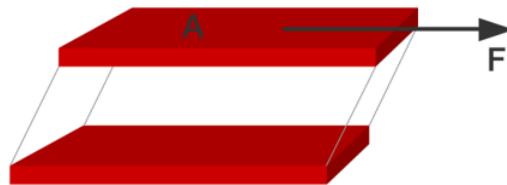
Figure 7. Shear stress is the force moving the upper plate divided by the plate's area [14].
