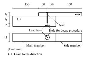
Fig. 3. Configuration of nailed connection specimen.
