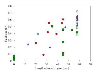
Fig. 10. Relationship between yield load and sound distance in boundary between main and side members. *Open circles*, control specimens of S3M7; *filled circles*, decay-treated specimens of S3M7; *open triangles*, control specimens of S6M4; *filled triangles*, decay-treated specimens of S6M4; *Open squares*, control specimens of S8M2; *filled squares*, decay-treated specimens of S8M2
