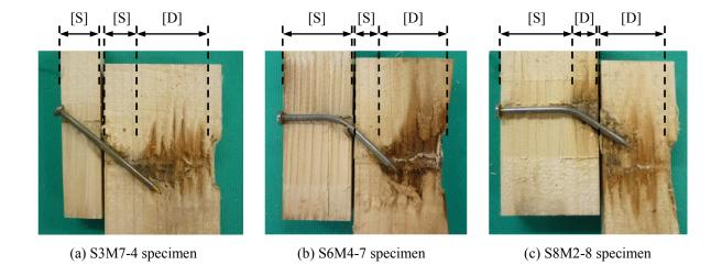
Fig. 7. Cross section of nailed connection after loading test.
