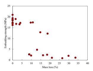
Fig. 6. Relationship between embedding strength and mass loss.
