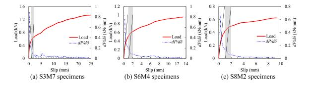
Fig. 9. Inclination of tangent of load-slip curves.
