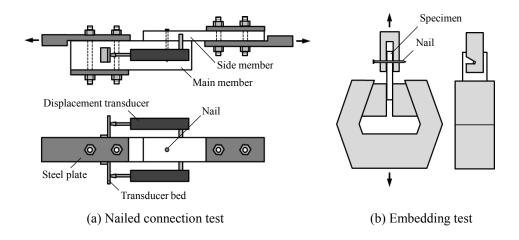
Fig. 4. Setup of lateral loading tests for nailed connection and embedding tests.
