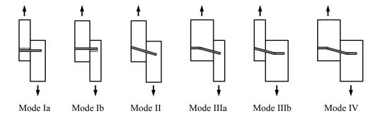
Fig. 2. Yield mode of nailed connection.
