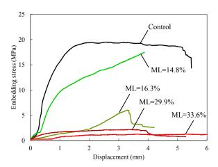
Fig. 5. Relationship between the embedding stress and displacement.  $ML,\, mass\, loss$
