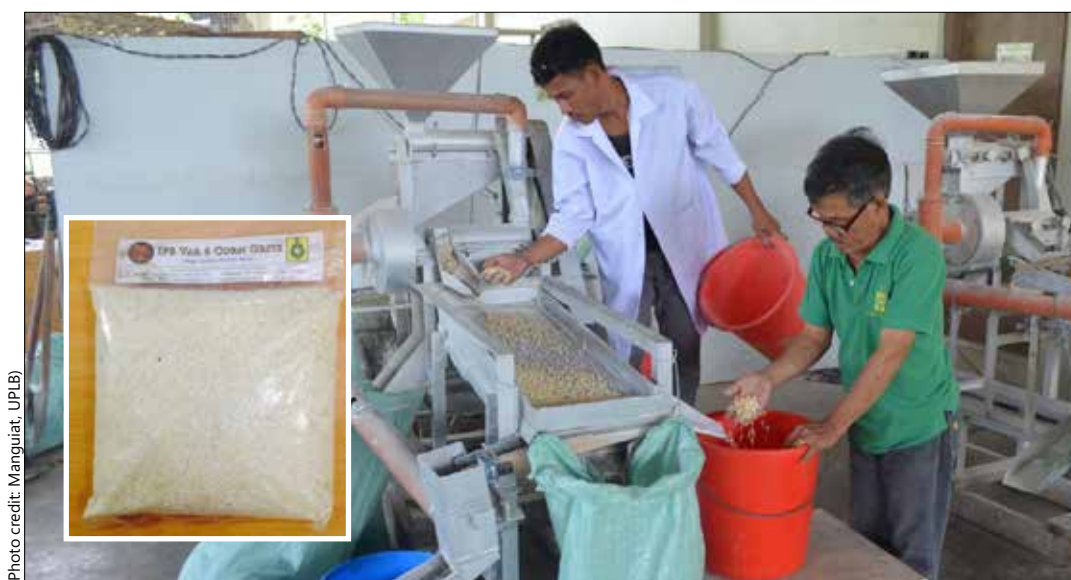
Figure 2.39. A village-type compact corn mill for white corn is used in corn grits production
