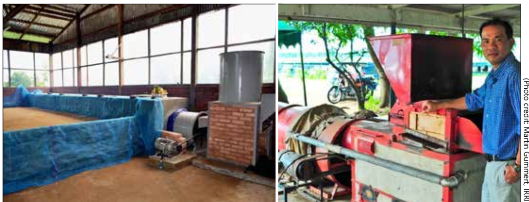
Figure 2.19. FBD with 4 t capacity and simple inclined grate rice husk furnace in Myanmar (L); Semi-automatic downdraft rice husk furnace (R)
