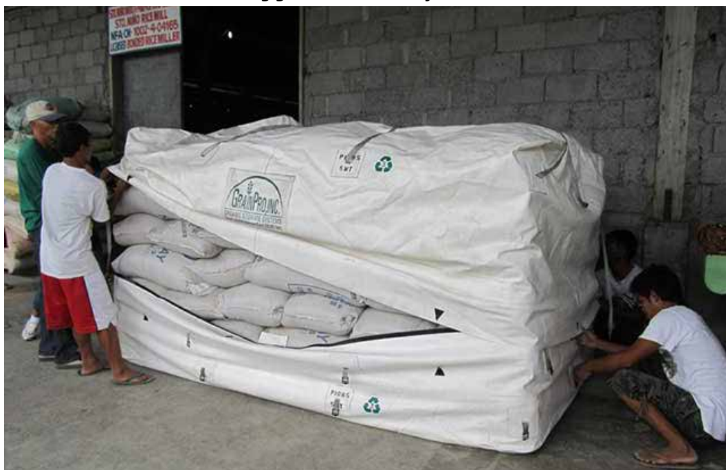
Figure 2.20. Hermetic grain storage in a Cocoon™, an airtight and pesticide-free method of storing grains and other dry commodities
