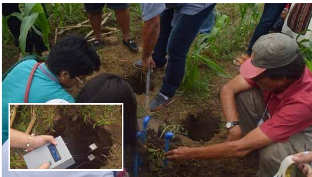
Figure 2.60. WAISS provides farmers with real-time soil moisture content data and immediate recommendations for irrigation schedule
