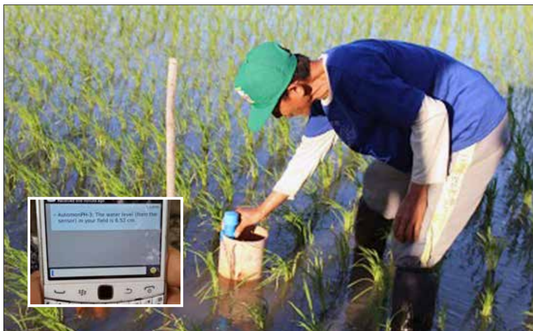
Figure 2.58. AutoMon is an ICT tool rice irrigation management
