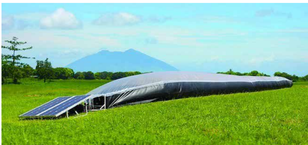
Figure 2.18. Solar bubble dryer is a drying technology developed by IRRI, Hohenheim University, and GrainPro
