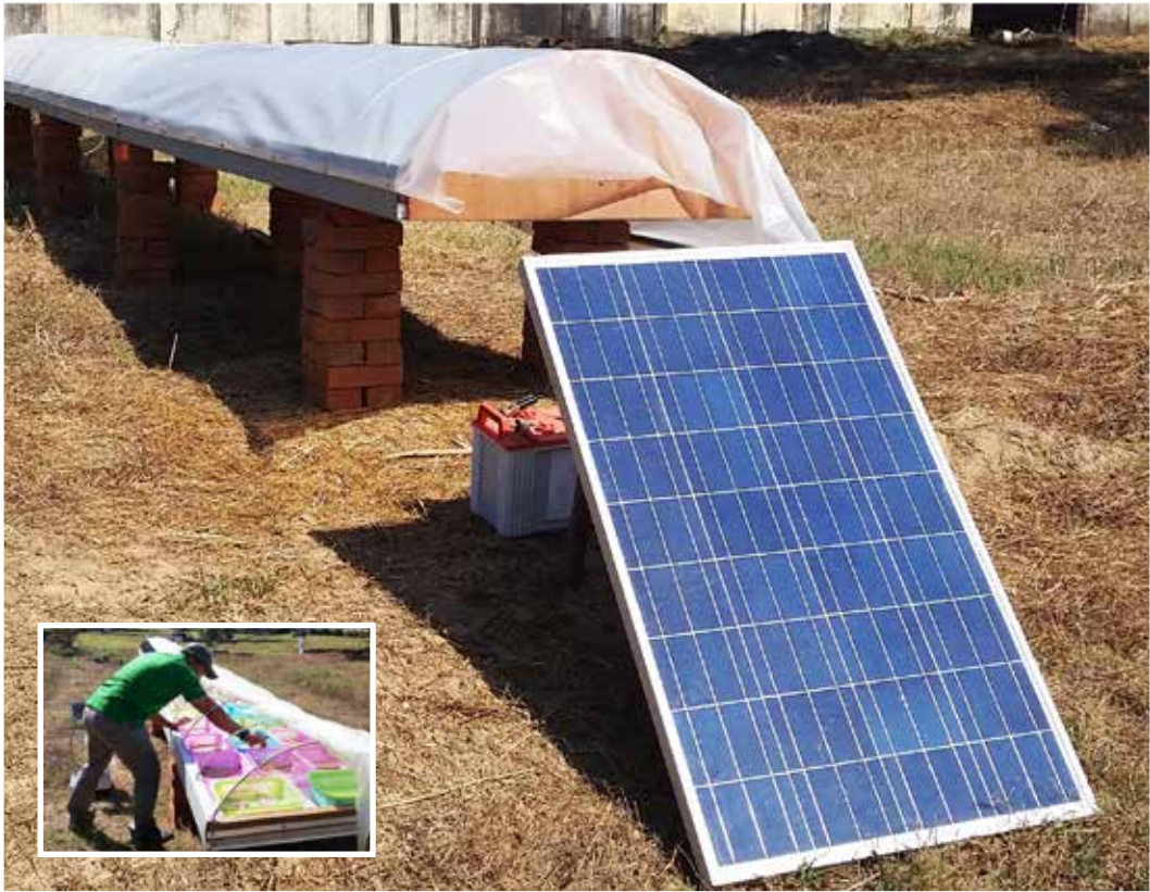
Figure 2.51. Solar tunnel dryers maintain the quality of fish products and other commodities while promoting energy conservation
