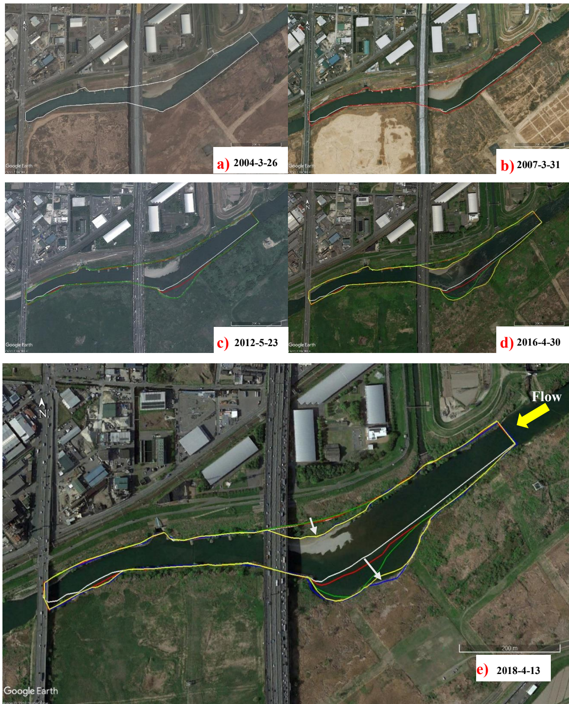
Fig.10 (a-e): Bankline change due to erosion of banks
