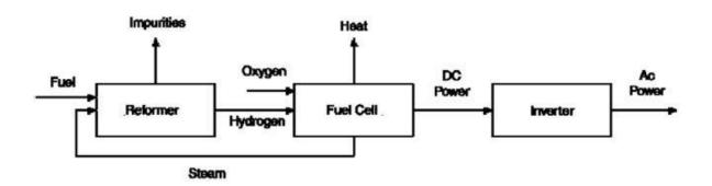
Figure 5.49 Simplified Schematic Plan of a FC utilizing Refined Hydrogen from a Reforming Unit
