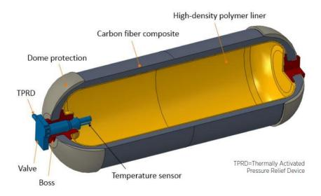
Figure 5.44 A schematic of a Composite overwrapped pressure vessel designed for compressed hydrogen storage onboard FCEVs [U.S. Department of Energy, 2018]
