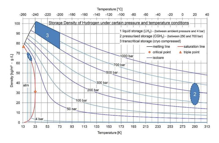
Figure 5.41 Net Storage Density of Hydrogen [Wikipedia, 2019]
