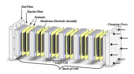
Picture 2.11 A typical Fuel Cell Stack
