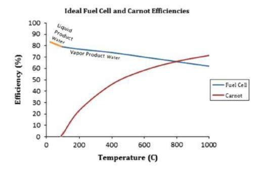
Figure 2.14 Comparison between the Thermodynamic Efficiencies of the Carnot and the Fuel Cell process
