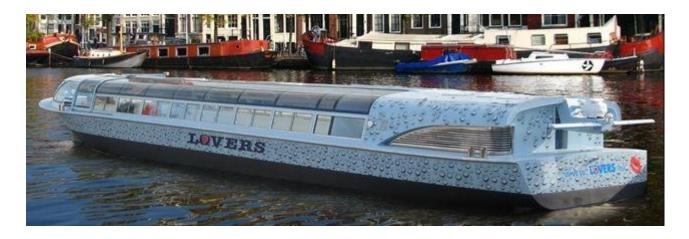
Picture 3.19 NEMO H2, the first fuel cell powered canal boat
