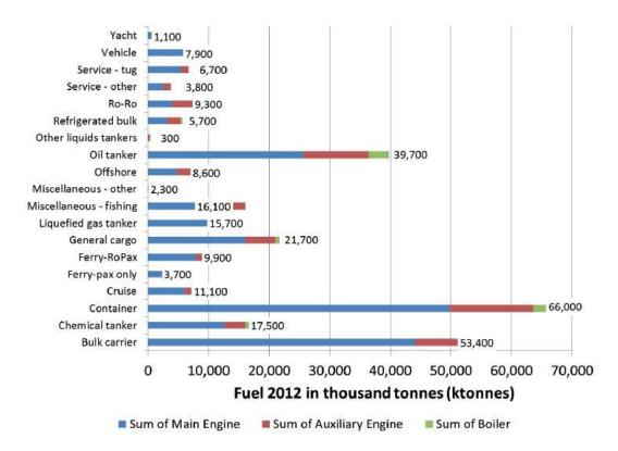
Figure 1.4 Summary graph of annual fuel consumption broken down by ship type and machinery component (main, auxiliary and boiler) in 2012
