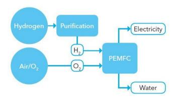
Figure 2.18 Schematic of a PEMFC
