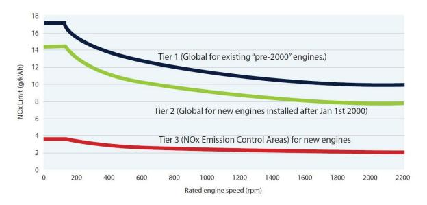
Figure 1.6 Regulations for NOx emissions for new-build ships in ECAs [ABS, 2018]
