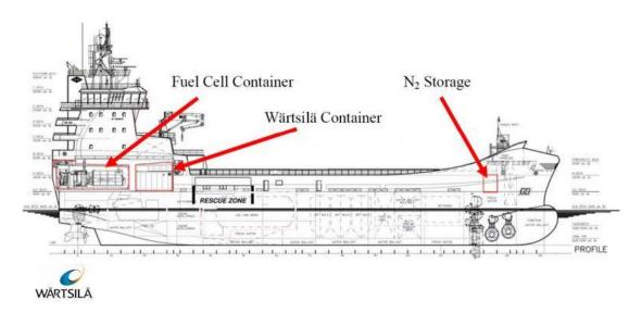
Figure 3.24 Layout of "Viking Lady's " fuel cell elements on board
