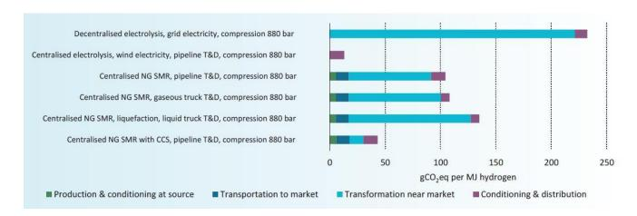
Figure 5.40 Today's carbon footprint for various hydrogen pathways in the European Union adapted from [Joint Research Center, 2013]
