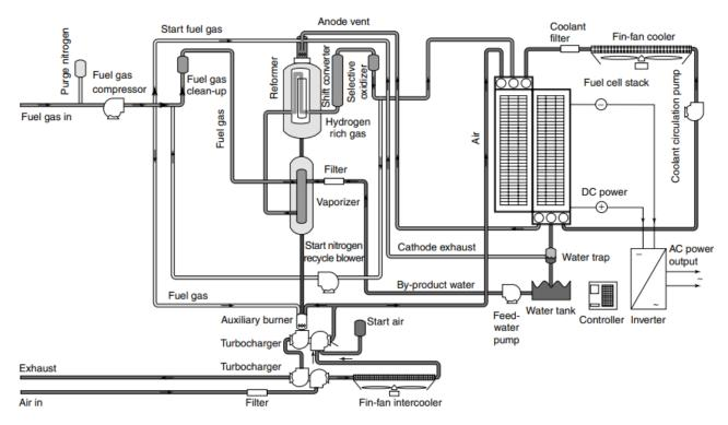
Figure 2.17 Process flow diagram for a Ballard 250-kW PEMFC plant [Source: Larmine and Dicks (2003)]
