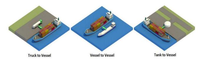
Figure 5.52 LNG Bunkering Options [Holden, 2014]
