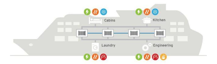
Picture 3.18 The Principles of a decentralized network with fuel cells supplying electric power
