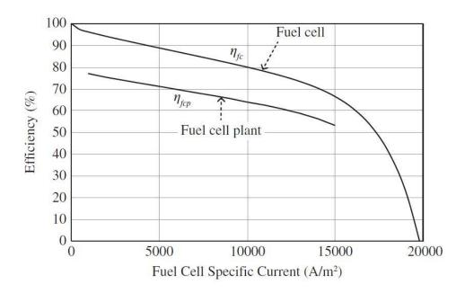
Figure 2.16 PEMFC total system efficiency curve
