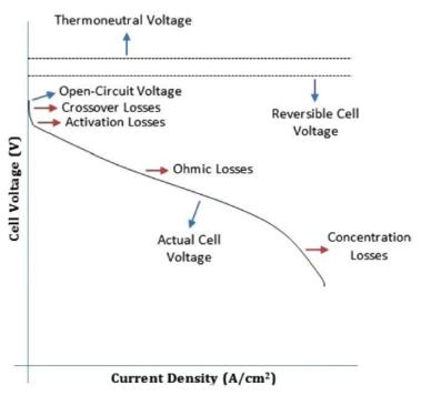
Figure 2.15 A Typical Polarization Curve with Voltage Losses
