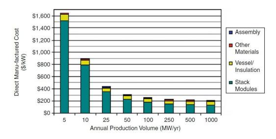
Figure 5.57 Manufacturing cost of planar SOFC Stacks (Economy of Scale in FCs Production) [IEA, 2015]
