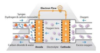
Figure 2.21 Energetic Flows in a SOFC
