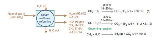
Figure 5.36 SMR block diagram and governing reaction [A.Scipioni, 2017]
