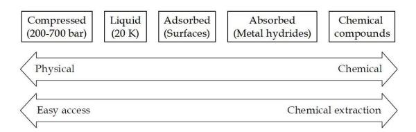
Figure 5.43 The sequence of hydrogen storage techniques from physical to increasingly chemical [Jens Oluf Jensen, Qingfeng Li and Niels J. Bjerrum, 2014]
