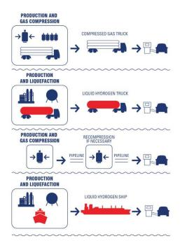
Figure 5.39 Delivery Paths of Hydrogen [Hydroville, 2019]
