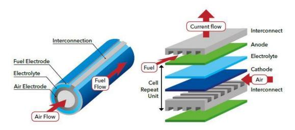
Figure 2.22 Cell structure of tubular (A) and planar (B) Solid Oxide Fuel Cell
