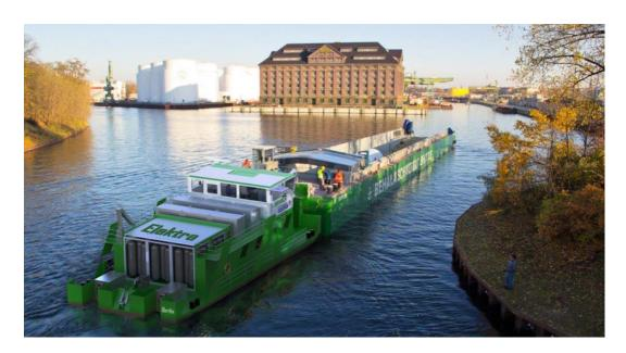
Picture 3.21 Elektra: a hybrid ship using FCS and rechargeable batteries
