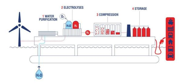
Figure 5.38 Schematic presentation of Water Electrolysis using Wind energy conversion [Hydroville, 2019]
