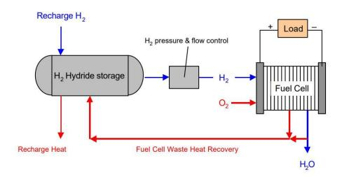
Figure 5.45 Example of a typical vehicular hydrogen fuel cell system. [Trygve Riis and Gary Sandrock, 2005]
