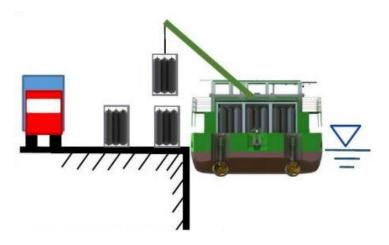
Picture 3.22 Elektra's proposed bunkering system
