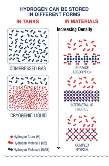
Figure 5.42 Hydrogen Storage Techniques [Hydroville, 2019]
