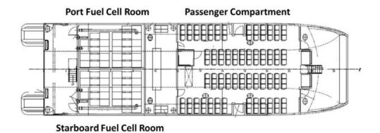
Figure 3.28 Cutaway view of the Main Deck of the SF-BREEZE. The PEM fuel cells are distributed into a Starboard Fuel Cell
