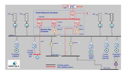
Figure 3.23 Fuel Cell integration in "Viking Lady's" electric propulsion system
