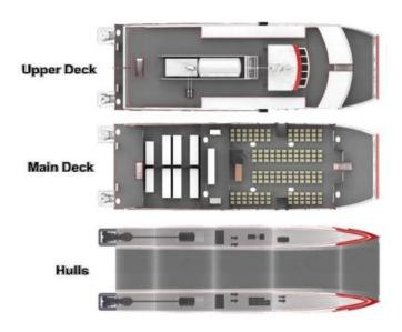
Figure 3.29 The three decks of SF – BREEZE
