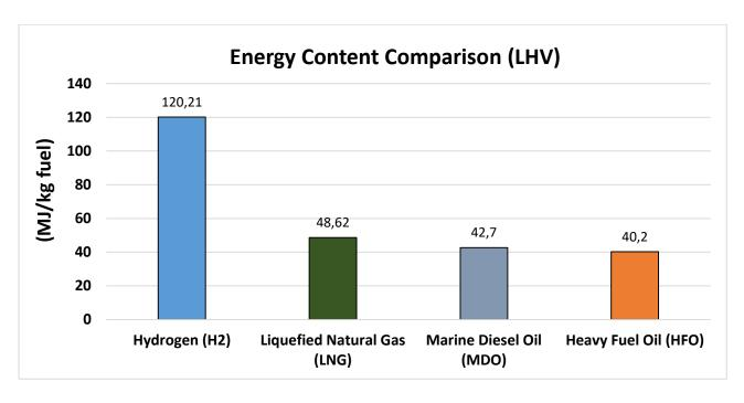
Figure 5.47 A comparison of energy content (LHV) between Hydrogen, LNG, MDO and HFO [DNVGL, 2018]
