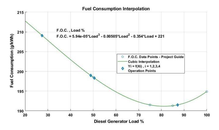
Figure 6.61 Fuel Oil Consumption [F.O.C.] calculation using Matlab Interpolation
