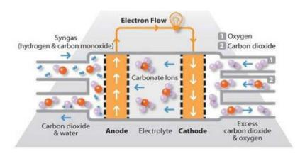
Figure 2.20 Energetic Flows in a MCFC
