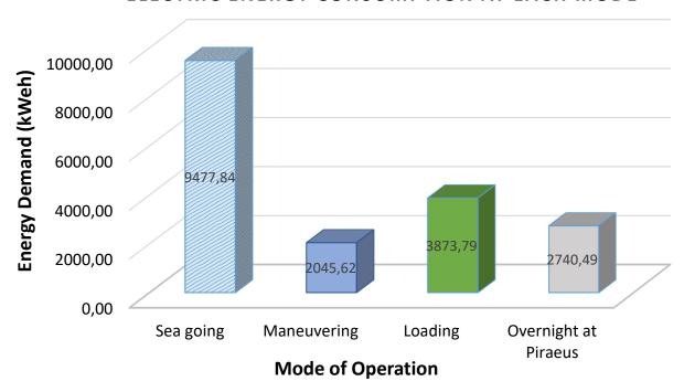
Figure 6.60 Blue Star Paros' Electric Energy Consumption at each Operation Mode for a Round Trip
