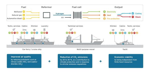
Figure 5.48 Fuel Cell Potential in Marine industry [e4ships, 2019]
