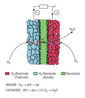
Figure 2.12 Layout of Fuel Cell's Electrochemistry
