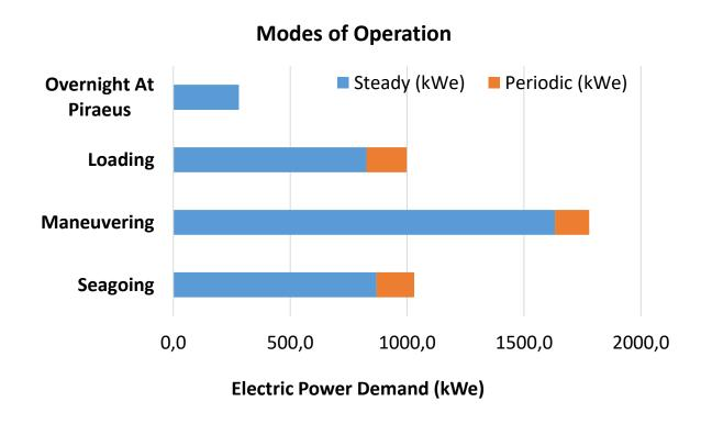
Figure 6.58 Blue Star Paros' Electric Power Demand in kWes for each Mode of Operation [Blue Star Ferries, 2019]
