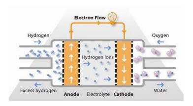
Figure 2.19 Energetic Flows in a PEMFC
