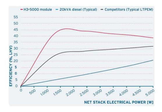
Figure 3.25 Typical level of efficiency of the Serenergy fuel cell and competing products
