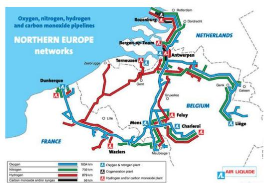
Picture 5.31 AirLiquide integrated pipeline network in the Benelux countries. Red lines represent H2 pipeline network. [AirLiquide, 2016]
