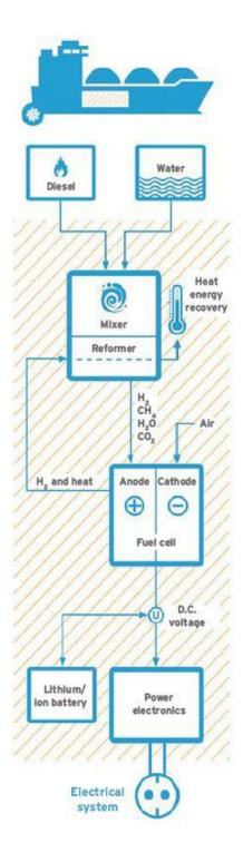
Figure 3.26 Hybrid Synergy of an electrical FC system [e4ships, 2019]
