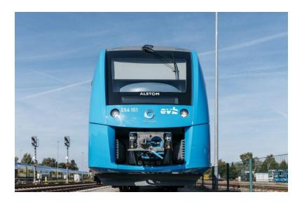
Picture 5.29 World's first hydrogen-powered fuel cell train operating in northern Germany [REUTERS, 2018]
