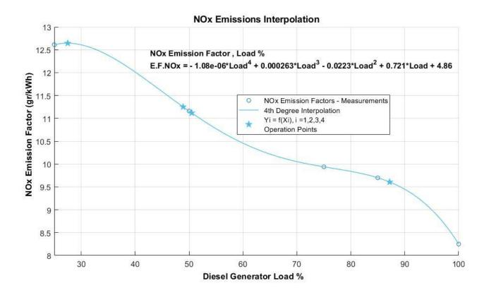
Figure 6.62 NOx Emissions Calculation using Matlab Interpolation
