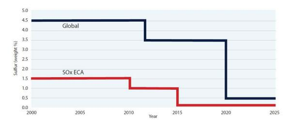
Figure 1.7 Present and future limits for sulfur content of marine fuel [ABS, 2018]
