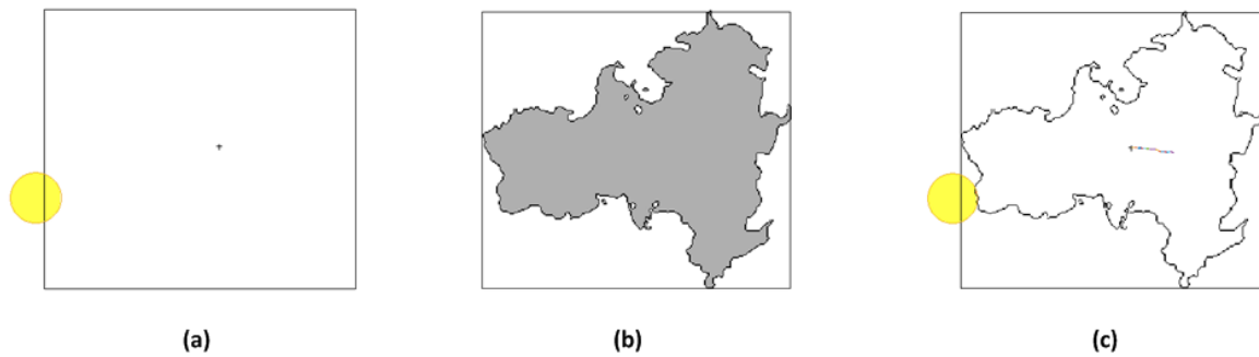
Figure 3.49 – Second example of cloud tracking and sun cover measurement.
