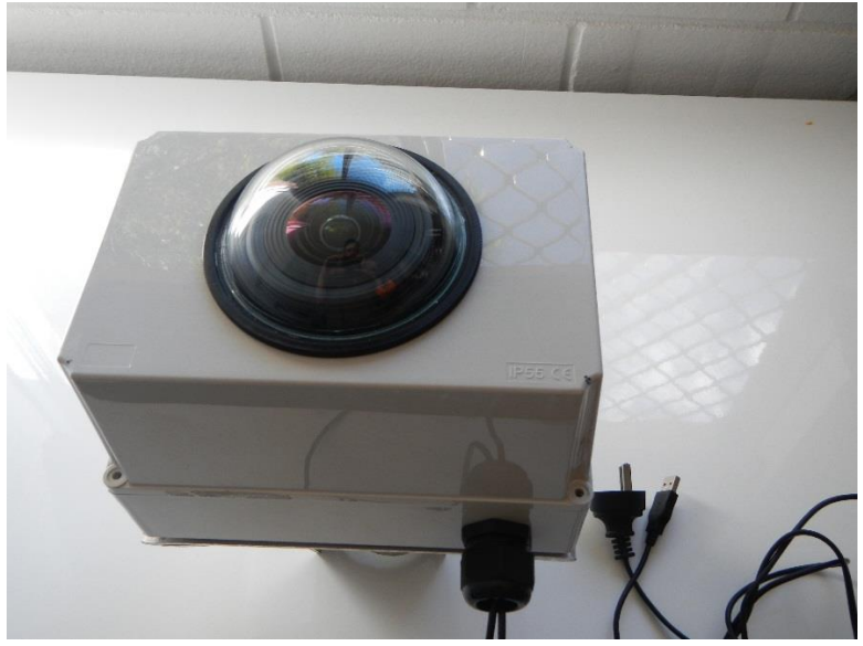
Figure B.3 – Camera box closed and ready to be installed.
