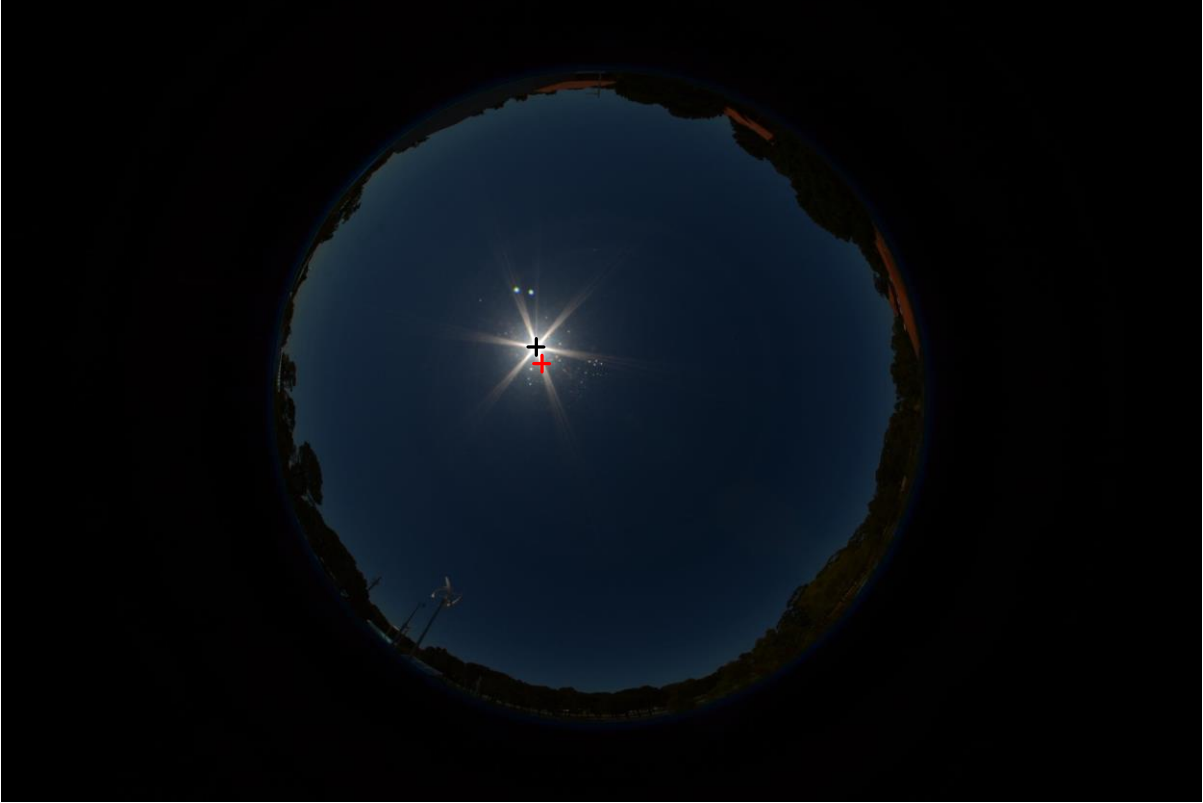
Figure 3.42 – Clear sky picture showing the position mismatch between predicted and actual projection of the centre of the solar disk.
