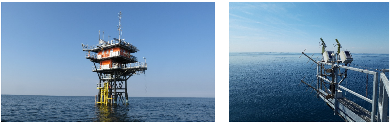
Figure 5. The AAOT site in the northern Adriatic Sea (left panel) and the dedicated AERONET-OC deployment structure (right panel) contemporaneously hosting 9- and 12-channel systems for data cross-comparison.
