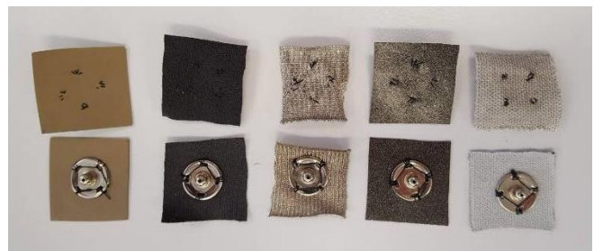
Fig. 1: Snap fasteners sewn onto material electrodes
