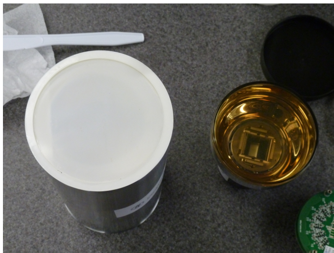
Figure 3.10: A \text{LaBr}_3(\text{Ce}) crystal (left) and photo multiplier tube (right).
