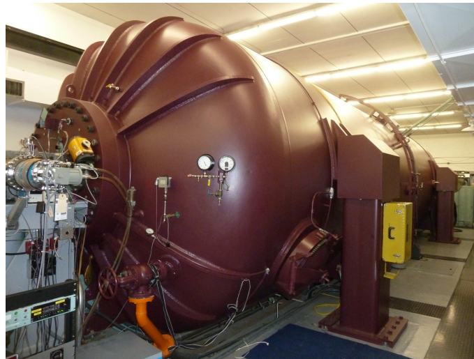
Figure 3.2: 9 MV tandem accelerator at John D. Fox Superconducting linear Accelerator Laboratory.
