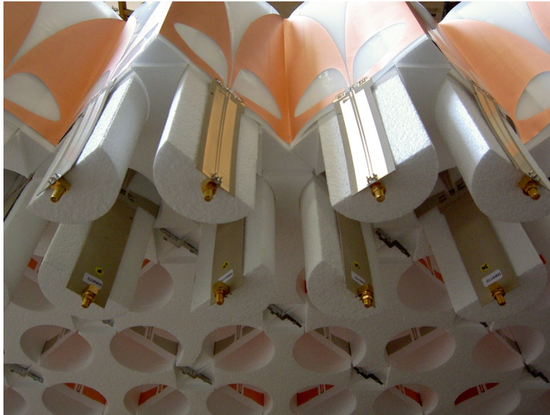
Figure 41 Foil based Vivaldi antennas in an EPS array
