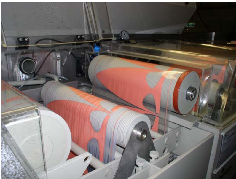
Figure 40 Copper plating screen printed Vivaldi antennas
