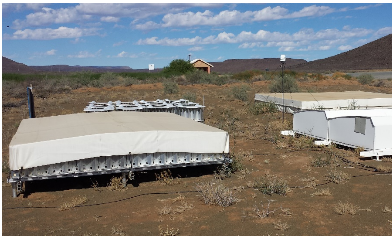
Figure 43 Local shielding, environmental proto types at the SKA site in the Karoo, South Africa
