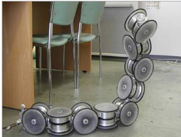
Figure 2.8. ACM-R4 with active wheels [65].
