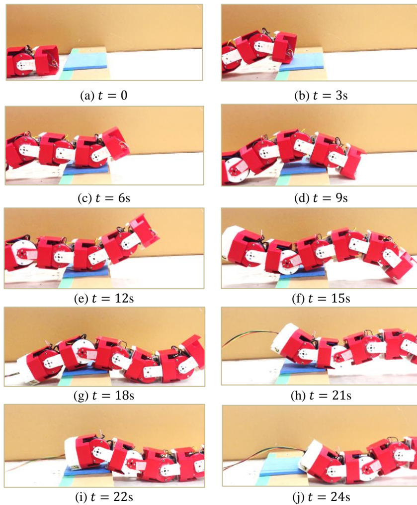
Figure 6.4. The robot climbing over an obstacle
