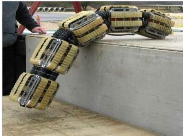
Figure 2.9. Omni Tread snake-like robot with active tread climbing over a stair [66].
