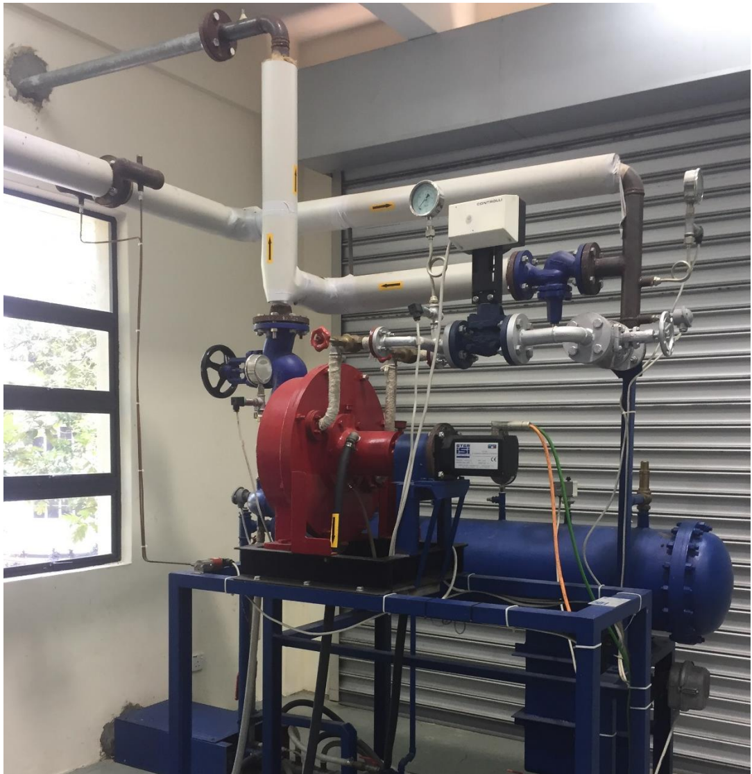
Figure 3.6: Turbine connected through shaft with generator
