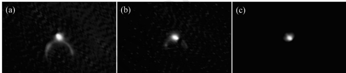
Figure 4.7: CCD images of the guided mode in (a) DRF, (b) single jacketed DRF and (c) double jacketed DRF.
