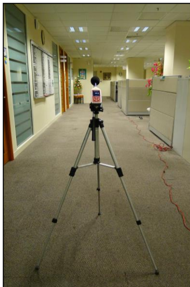
Figure 3.13: The Cirrus in position during BN level measurement
