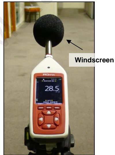
Figure 3.9: Cirrus Research CR:172B Optimum Green SLM (Cirrus)
