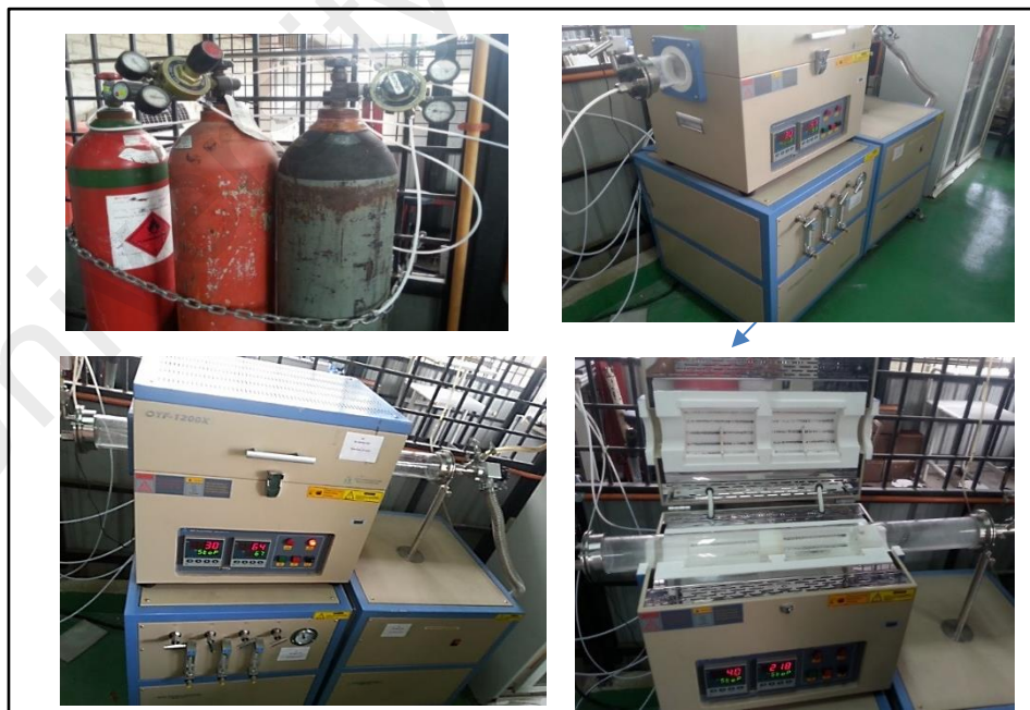
Figure 3.1: Photograph of the in-situ CVD reactor.
